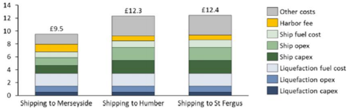
Figure 32: Unit costs of shipping CO2 from South Wales (undiscounted)
