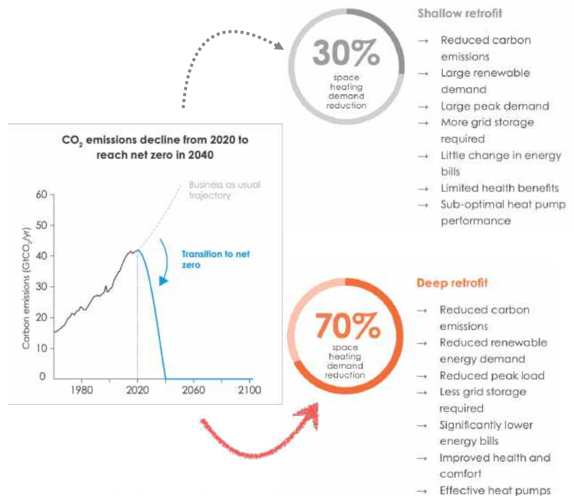
Figure 1.12 - Comparison of percentage of energy demand reductions and associated co-benefits from shallow and deep retrofits.
